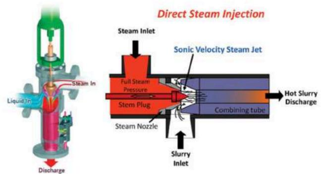
*SHEAR POWER: The patented Hydroheater combines steam with mechanical shear to heat and open the starch molecule for enzymes to do their work.*
