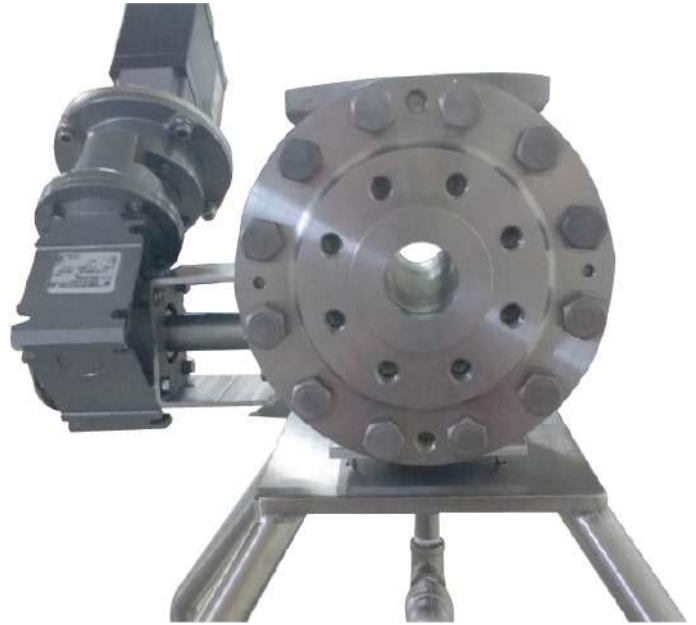
The straight-through design of the NOH.
