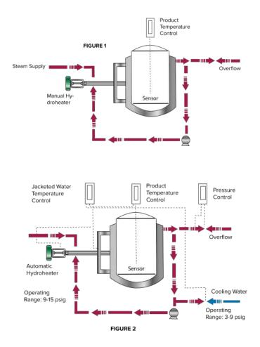
temperature following the set point as rapidly as changes are called for by the master batch Temperature Controller. Steam flow is controlled from 100% flow for maximum "come up", down to "no flow" during cooling periods. The precise temperature control obtained has enabled users to operate at optimum temperature conditions to obtain the greatest yield from the batch.
